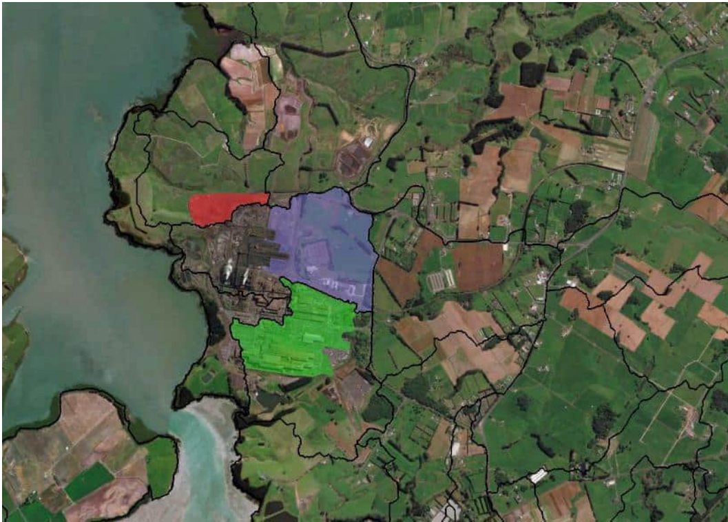
Figure 4-5. Catchment areas used to adjust the FWMT flow and load data for the Waitangi Stream 3 (blue), Waitangi Stream 4 (red) and Waitangi Stream 6 (green) nodes based on operational data from NZ Steel. Adjustments to the FWMT Waitangi Stream 5 data accounted for on site processing of flows and the analysis of the Northside and Southside Outfall data.
